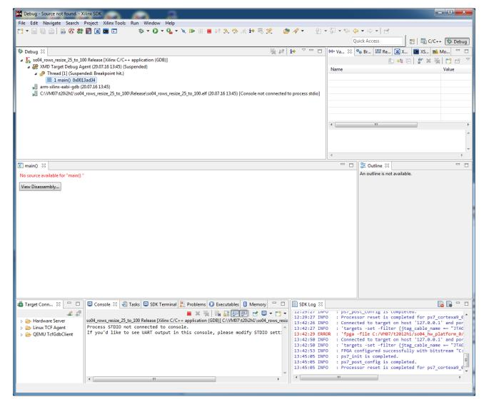
Figure 22: Debug stops at first executable line of ARM Cortex A9 code.
