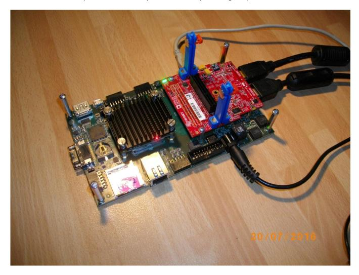
Figure 1: TE0701-05 platform with Zynq XC7Z020-2I device and HDMII-HDMIO support.
