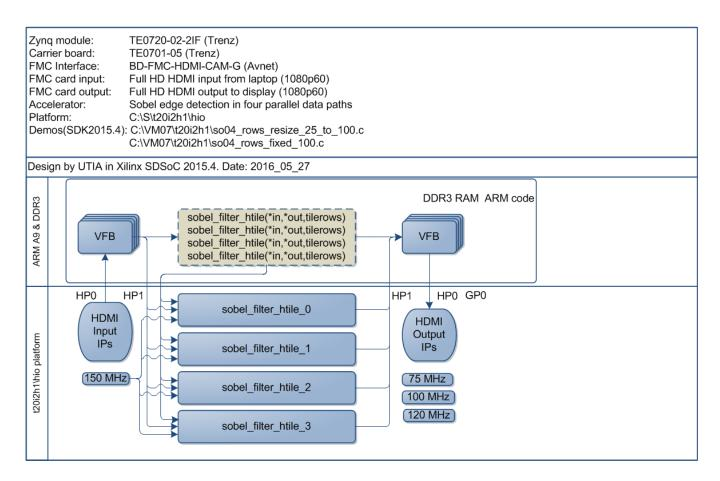
Figure 9: Project so04 – Alternative programming style - Edge detection with four HW accelerators.
