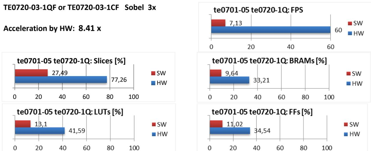
Figure 8: Project sh03 - Acceleration and HW resources used.
