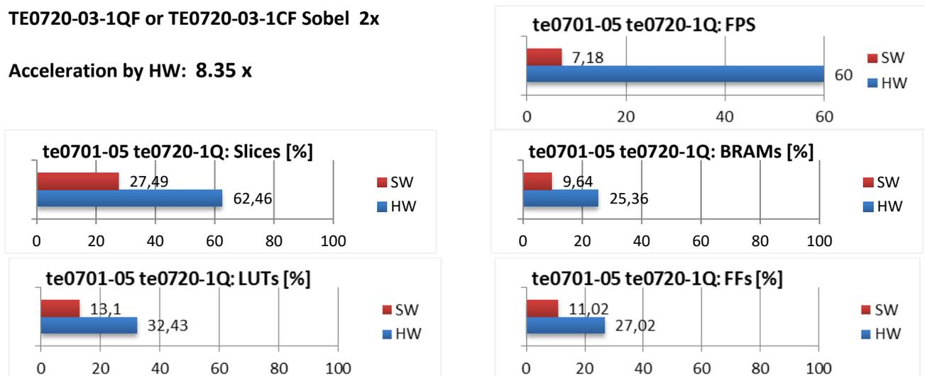
Figure 6: Project sh02 – Acceleration and HW resources used.
