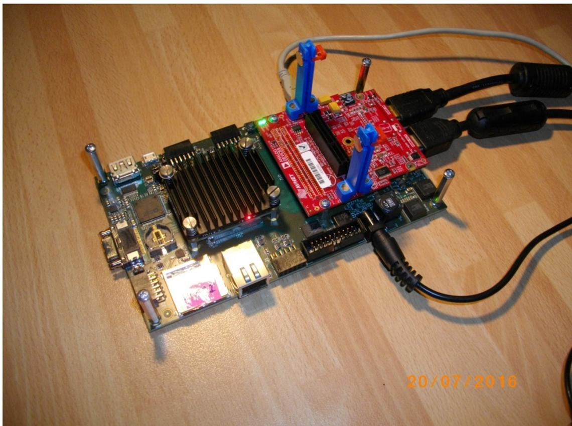
Figure 1: TE0701-05 platform, Zynq device and HDMII-HDMI support.
