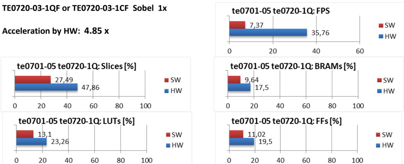
Figure 4: Project sh01 - Acceleration and HW resources used.
