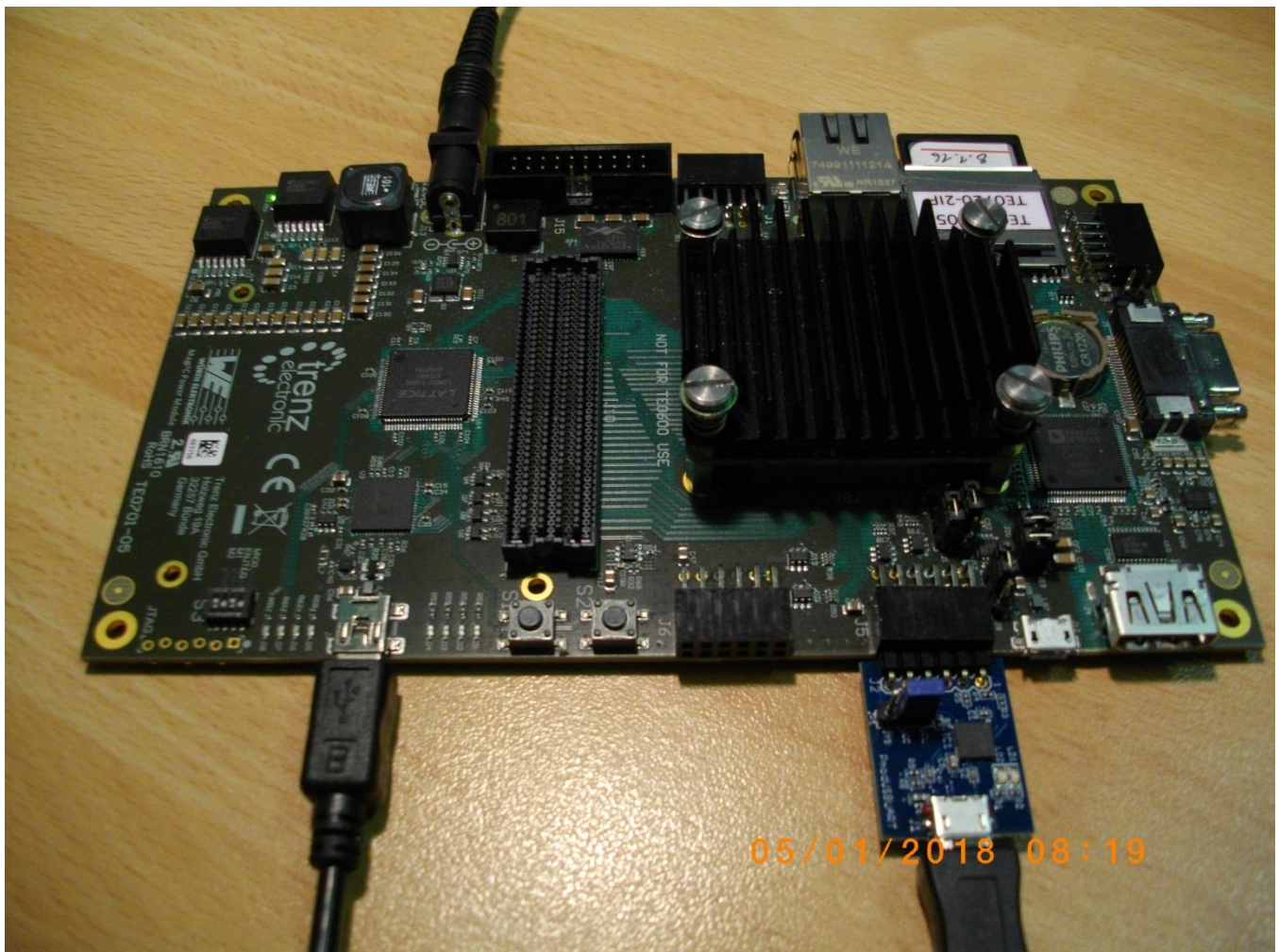
Figure 6: MiniUSB cable and MicroUSB cable for the Pmod USBUART
