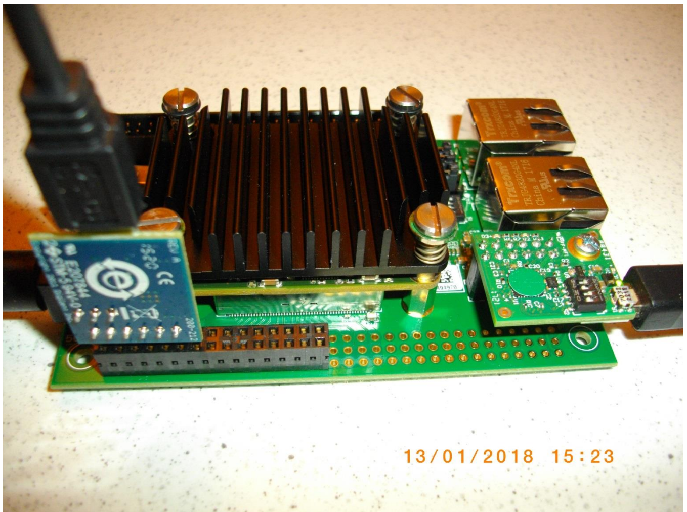
Figure 5: MicroUSB cable: Pmod USBUART. MiniUSB cable: XMOD FTDI JTAG adapter.
