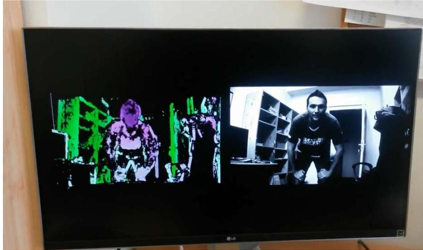
Figure 6: Sample Stereo Demo output, hardware accelerated video processing 23.5 FPS.
