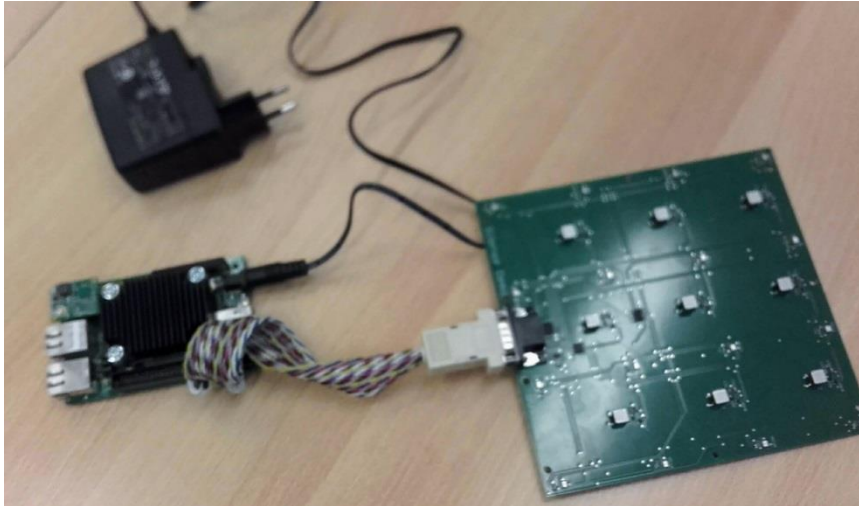
Figure 1: Hardware setup: Carrier TE0706, module TE0720, XMOD FTDI JTAG Adapter TE0790, passive heatsink, BUT mic array prototype, connection cable and power source.
