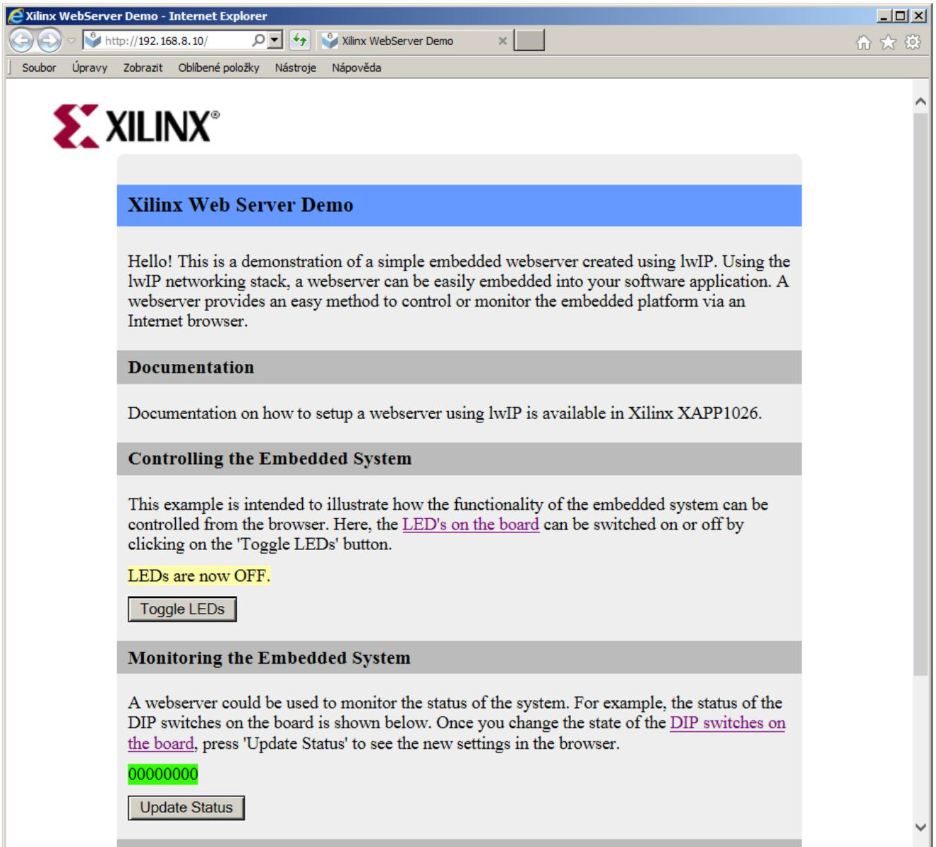
Figure 24: The demo www server is evaluating the basic GUI for communication from the web browser client to the Artix7 application working as an embedded server providing 1 G bit point to point connection.
