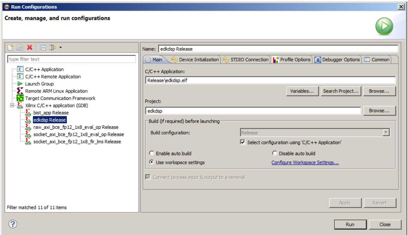
Figure 52: Recompile edkdsp project, download the .bit file and run the edkdsp.elf on Artix.
