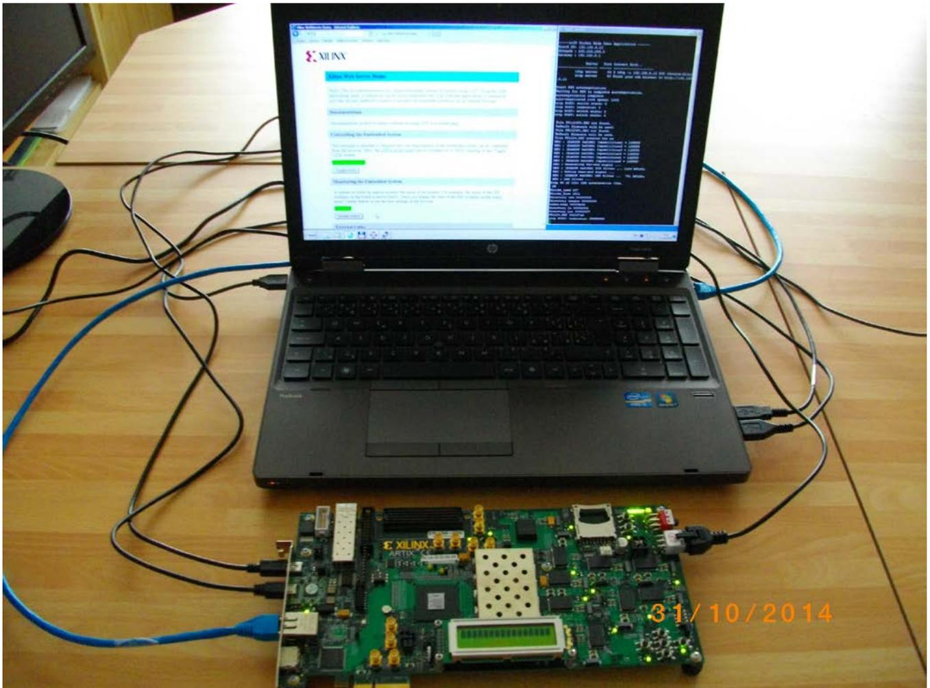
*Figure 1: Demonstration of IoT application combining the 1 Gb ethernet, www server and TFTP server with 6x (8xSIMD) EdkDSP floating point accelerators on Xilinx AC701board with Artix7 FPGA.*
