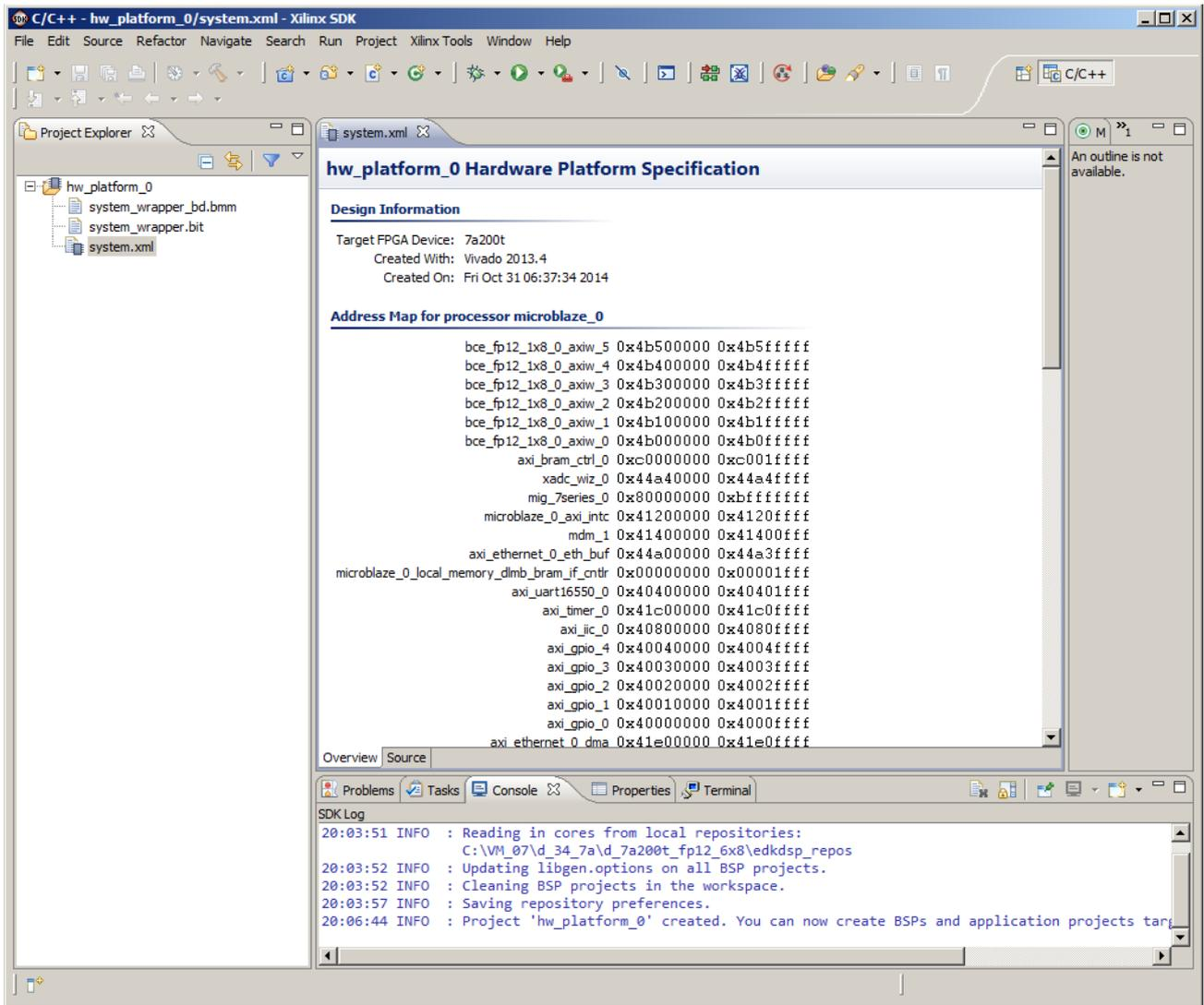
Figure 9: Hardware platform with the MicroBlaze processor and the address map
