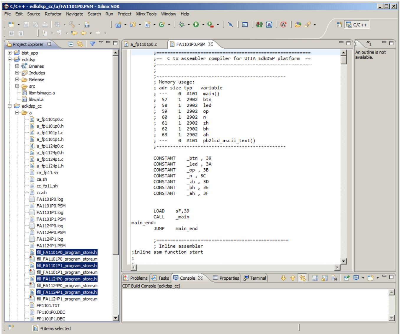
Figure 49: Select firmware header files and Ctrl-C Ctrl-V them to the edkdsp/src directory.
