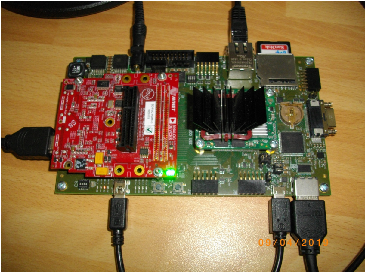
Figure 1: TE0820-03-4EV-1E on TE0701-06 carrier with Imageon HDMI I/O FMC card
