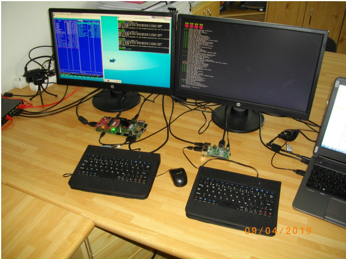
Figure 2: The Zynq Ultrascale+ TE0820-03-4EV-1E module and RaspberryPi 3B
