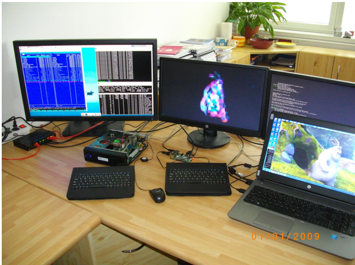
Figure 13: HW accelerated LK DOF input/output Full HD HDMI 60 fps
