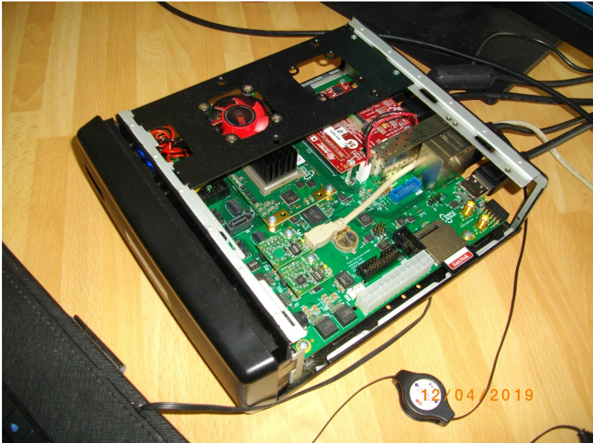
Figure 1: TE0808-03-15EG-1EE on TEBF0808-04 carrier with Imageon HDMI I/O FMC
