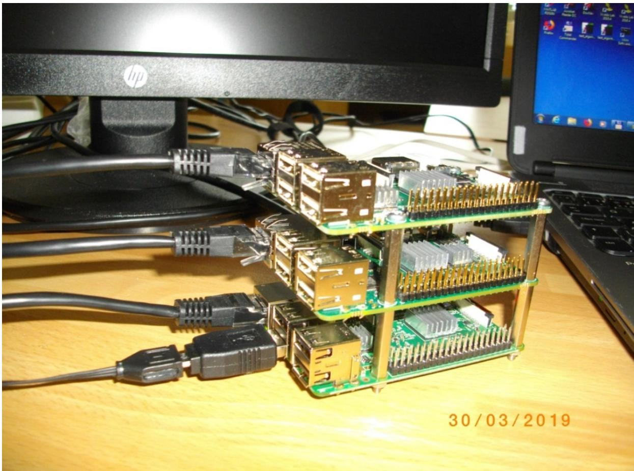
Figure 3: RPi3, Arrowhead G4.0 clients on two ZynqBerry boards
