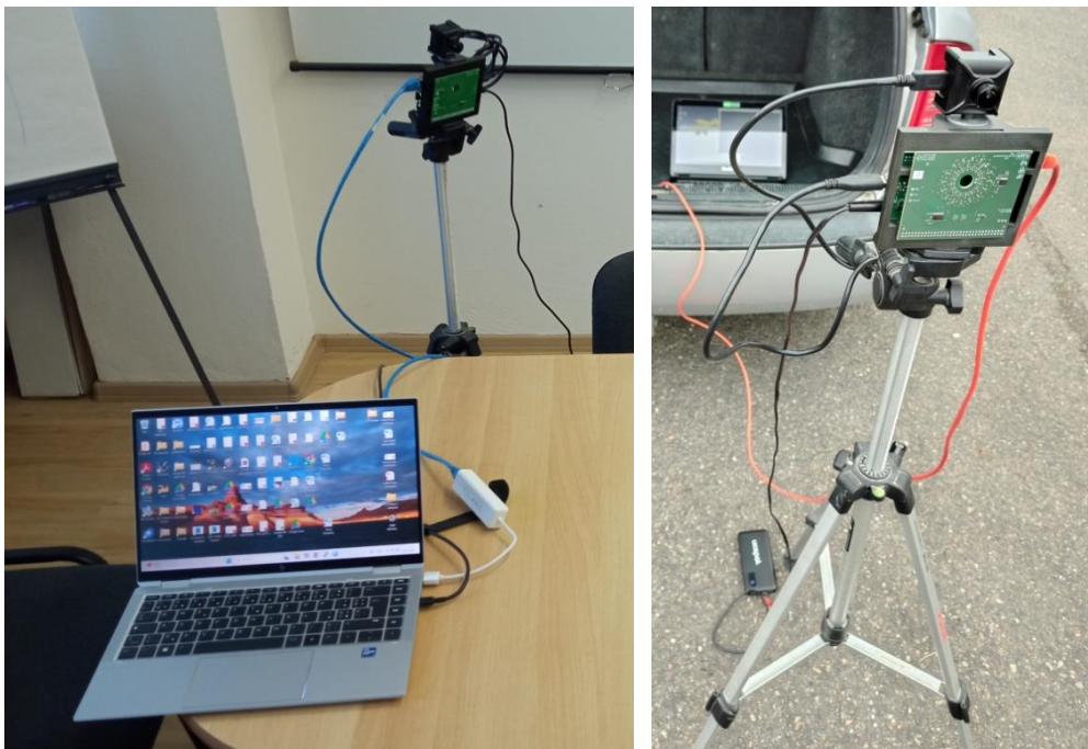
Figure 2: Examples of capture setup. The UTIA platform with microphone array facing front is mounted on tripod, powered and connected to PC using Ethernet.
